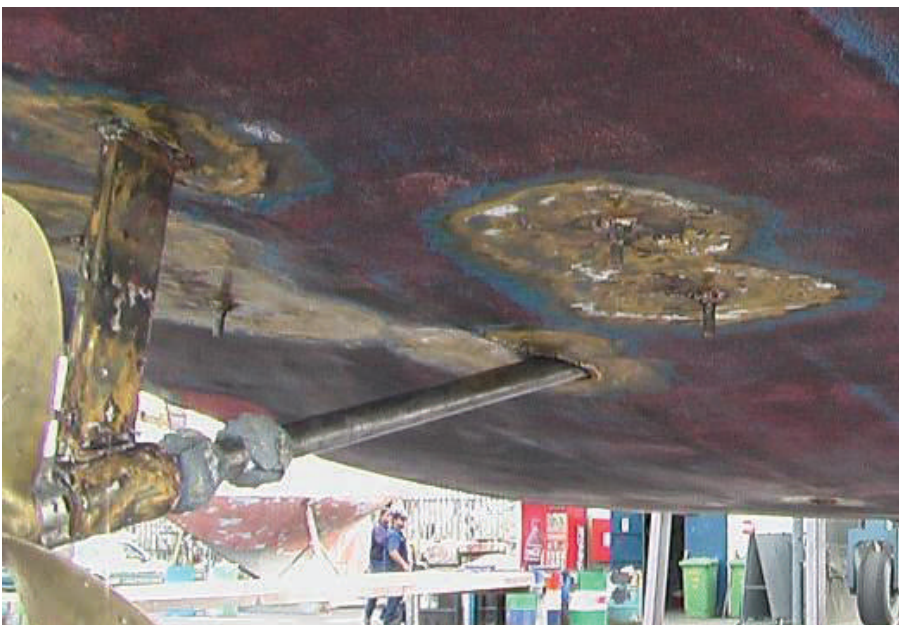
Paint blistered off around anode bolts, stern tube and P bracket
